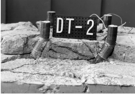
Figure 11 Test specimen loaded by shear force [6].
